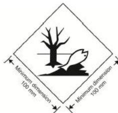
Figure 2-7: Environmentally hazardous substance mark
