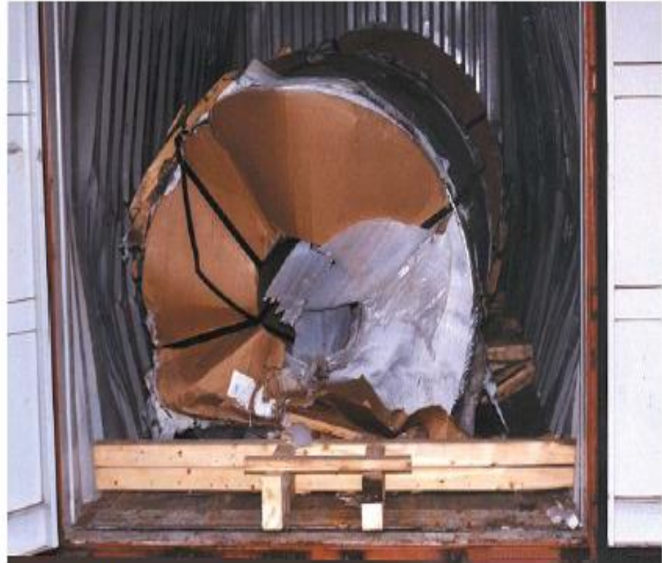
Photo 3. Note the damage caused to the container by the poorly secured coils
