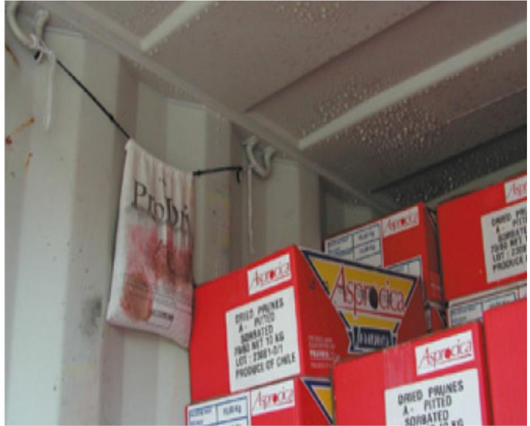
Condensation water on roof, dry bag already completely soaked
