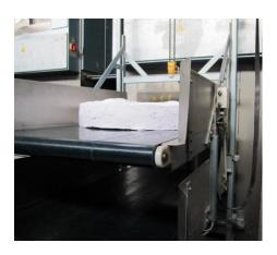
folding area. Whilst sheeting is not usually dried in the tumbler dryer, with a continuous batch washer, the "pancake" of sheets is placed briefly (approximately ten minutes on a low temperature) into the dryer to break up and loosen the sheets. From here all sheeting is then directed to the finishing area for folding or ironing and final processing.
